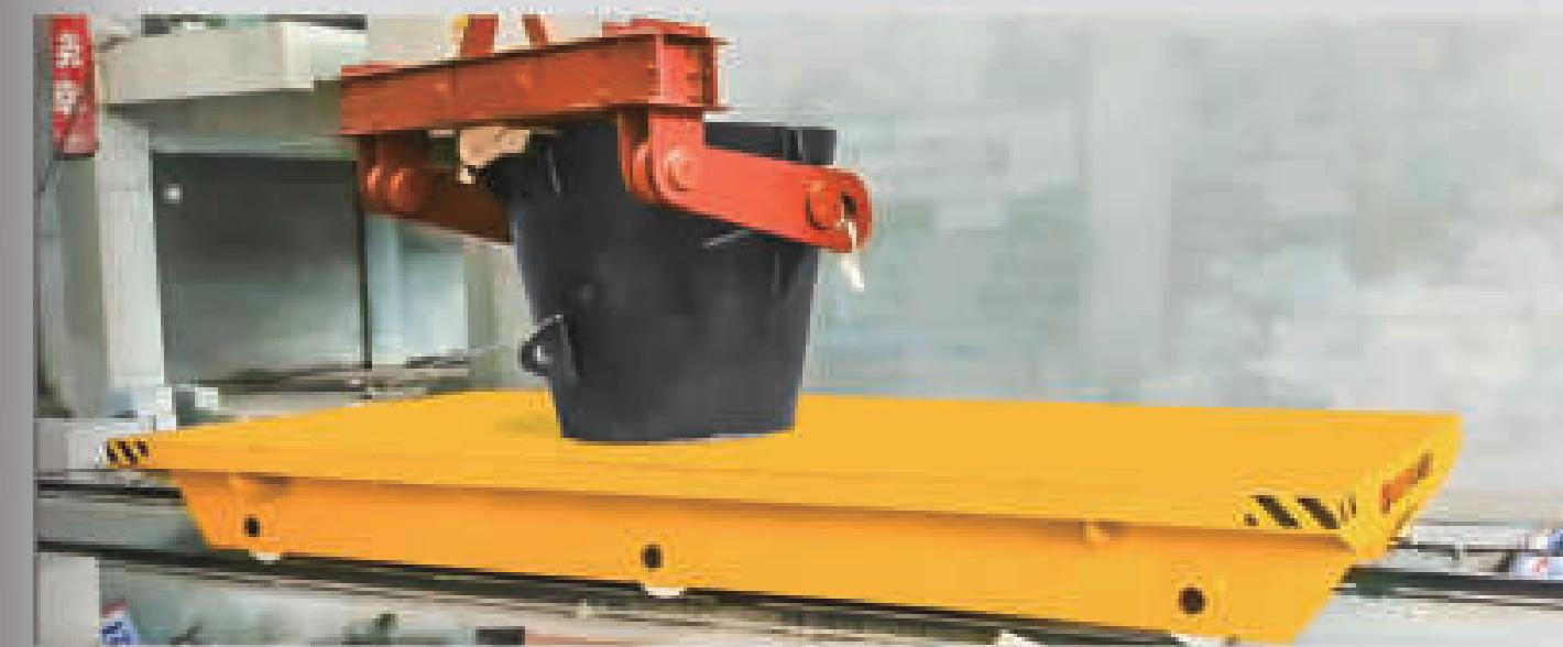
KP series unpowered rail transfer carts, also known as "rail trailers", "rail trolleys", and "human powered rail trolleys", are a transfer cart that running on the rails without power by themselves and are driven or towed by manual or other external forces (winches, forklifts, etc.). it is generally used in occasions with small load and short-distance transportation of materials. The towing device is a towing bar or towing hook.
