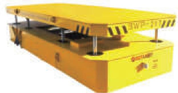
Hydraulic lifting transfer cart is a handling equipment with a hydraulic lifting device, which can raise the height of the lifting plate through the hydraulic cylinder, and then the workpiece is transported by the transmission belt to the designated assembly line or shelf.
