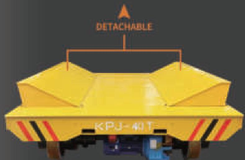
The electric transfer cart which has the 'U' frame is specially designed to transport the cylindrical workpiece which is easy to roll and drop.
