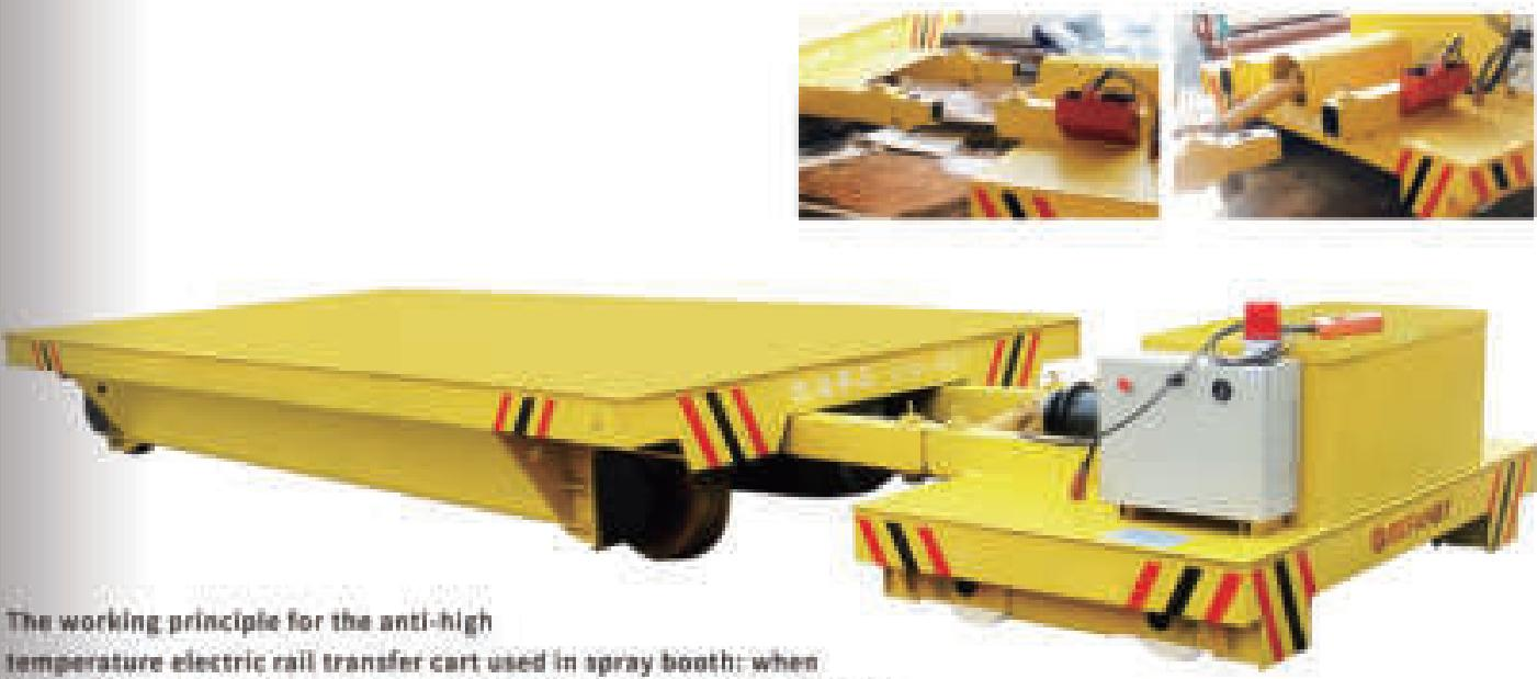
The working principle for the anti-high temperature electric rail transfer cart used in spray booth: when the whole cart runs into the spray booth, it is separated into two parts. The electric towing part runs out of the workshop which avoided the high temperature's influence to the motor, gear reducer and so on.
